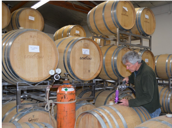
We gently push the wine out of barrel with nitrogen gas rather than use pumps which can introduce more oxidation.
